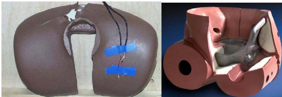
Figure 5: Shoulder foam cap with damaged skin (left), cut through a pelvis (right).
