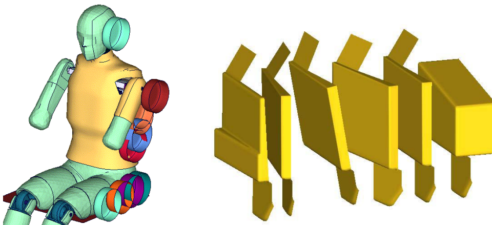
Figure 11: Pendulum impact locations (left) and barriers (right) used in tests for validation of ES-2 model.
