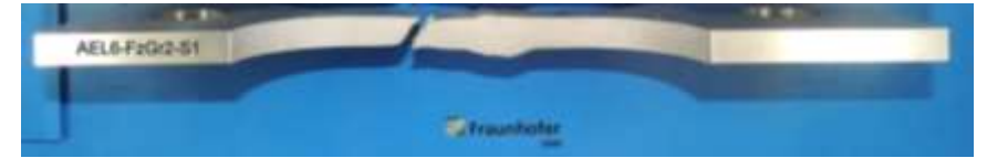
Specimens "as welded" fractured in softened HAZ
