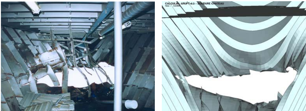
Figure 7 Rupture observed in the colliding bow
