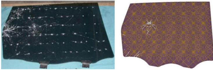
Fig. 16: Real and simulated material failure for the frame tests.
