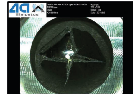
Fig.2: Highspeed video of a Puncture test
