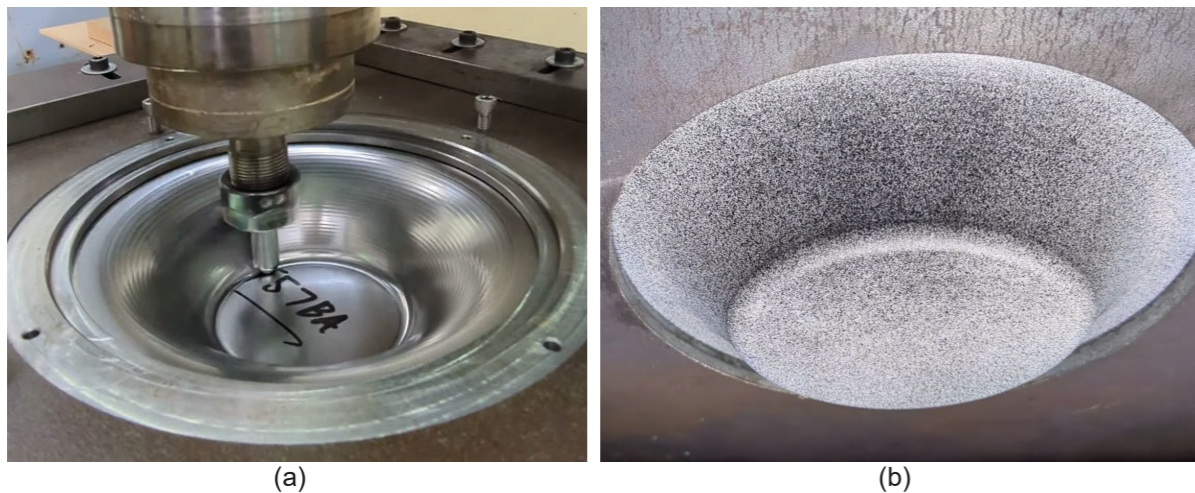
Fig. 1: (a) a partially formed SPIF specimen and (b) the underside of the specimen with speckle coating for DIC.
