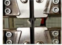
b: Compression Test ISO14126:1999
