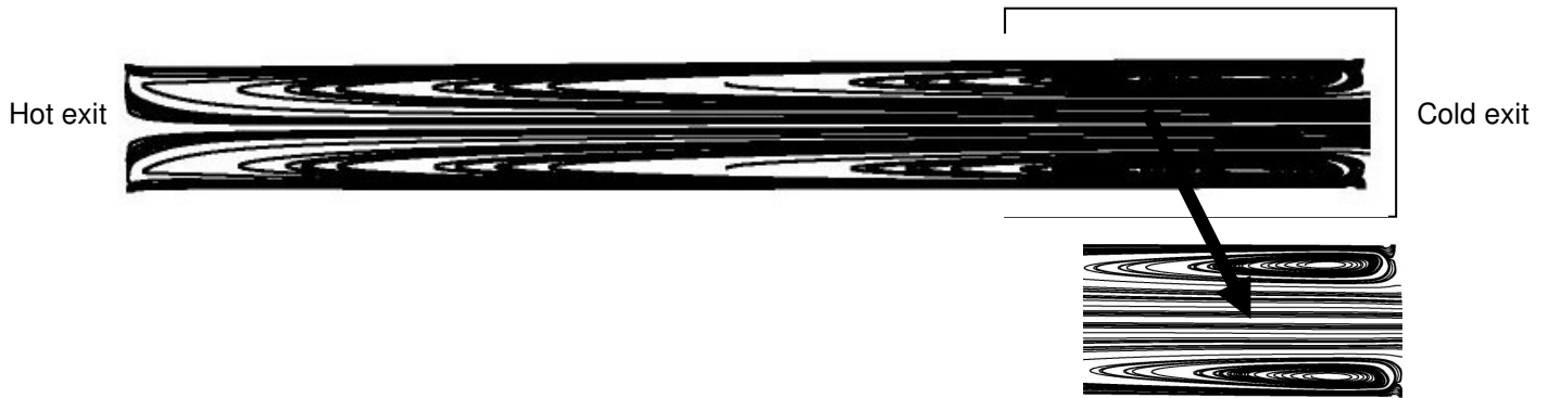
Fig.7: Flox field inside Conical Vortex Tube
