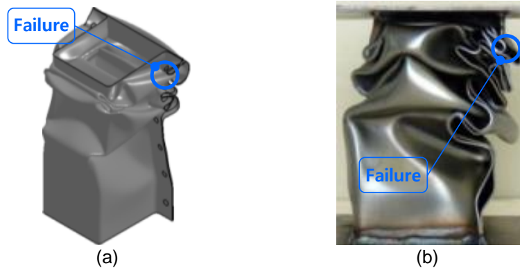
Fig.9: Deformed shape of the rectangular hat specimen: (a) simulation; (b) experiment
