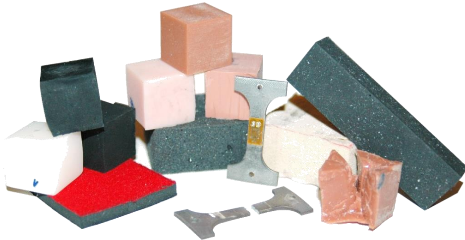
Fig.3: Material specimens of the WorldSID 50%.
