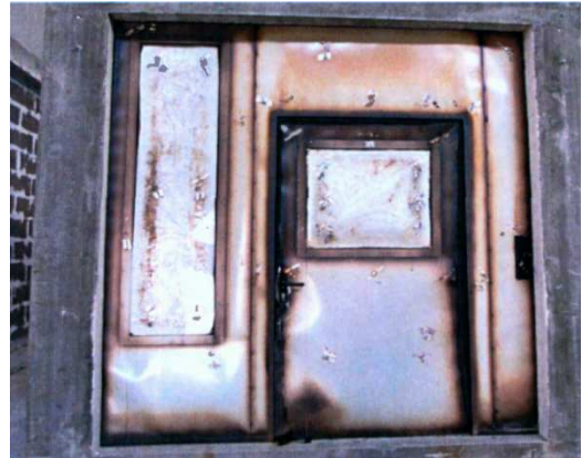
Fig.5: Specimen barrier - Unexposed side @90minutes
