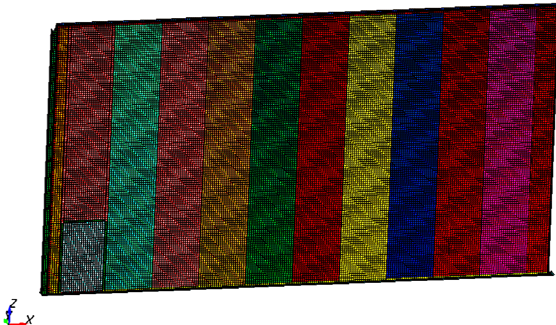
Fig.3: Example of Finite Element model of an enlarged fire door (wall opening dimension: 15000 x 8000 mm)
