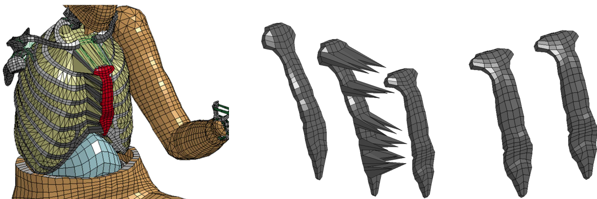
Figure 12: Results of step 1 – adaptation of the sternum (left) nodal motions of various sternum nodes and result, (right) comparison between kriging and cubic RBF interpolation
